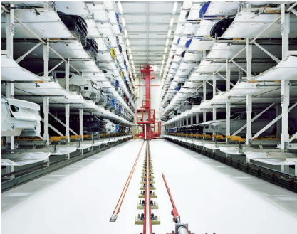
RIGHT Freshly painted car bodies are stored on huge shelves awaiting inspection before they can move along the production line
